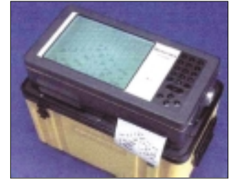
Geometrics SMARTSEIS 12 Channel Seismograph - The Geometrics Seismograph can be used for both seismic refraction and reflection surveys for shallow engineering exploration usually to 30 meters.
