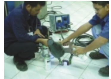
MAGNETIC PARTICLE TESTING
