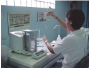
Volumetric Calibration using a Sartorius Microbalance
